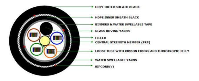
**3.9.1 Secondary Protection:** The primary coated Ribbon fibres may be protected by loose packaging within tube, which shall be filled with thix otropic jelly. The dimensions of tube shall be as per Table – I above.
