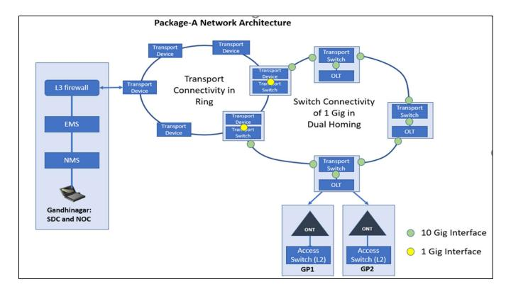
Note: 20 GP(Gram Panchayat) connected from 1 OLT(Optical Line Terminal) with 2 GP per PON(Passive Optical Network) Port of OLT, However, in OLT approximately 25-27 GPs Connected
