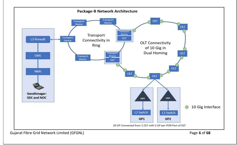
3.3 In a present network, physical connectivity between 2 layers of transport mux and transport switch/OLT is as per below in both packages.
